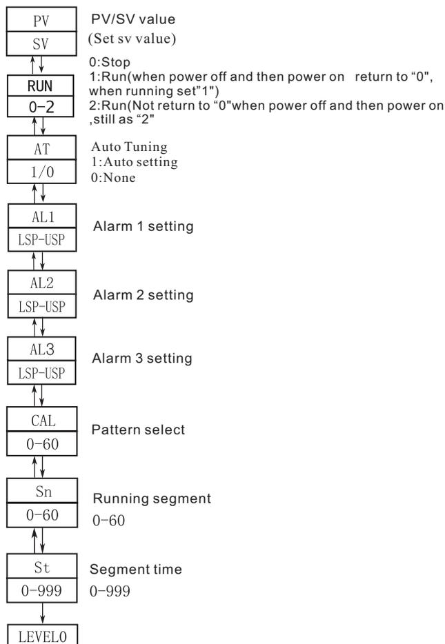
**LEVEL2** Control Program setup level (Engineer operation level)
